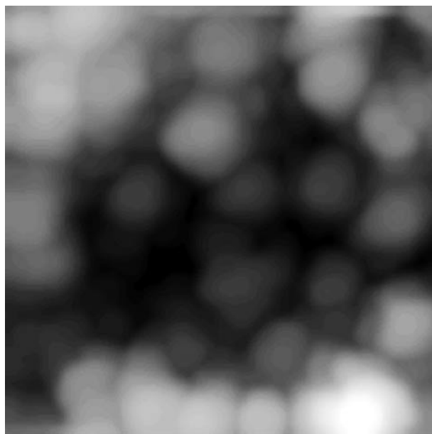
Figure 1. STM image ( 19.5 \times 19.5 nm) of 2–4 Ohm cm n-type (100) porous silicon surface in vacuum before heating. Constant current mode, tip voltage +1.28 V, current 1.12 nA.
